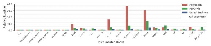
**Figure 9.** Runtime of the instrumented programs relative to the uninstrumented runtime, per analysis hook. Results are averaged over 20 runs (and again for readability, over the 30 PolyBench programs).
