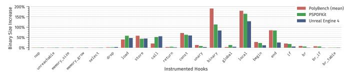
**Figure 8.** Binary size increase in percent of the original size, when instrumenting the test programs for different analysis hooks. For readability, binary sizes for the 30 PolyBench programs are shown averaged.
